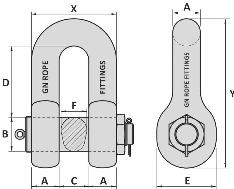
Dimensions for shackles are calculated by multiplying the common link size by the factor shown below
